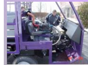
Full access to the engine for service is provided by rolling the cab forward .
