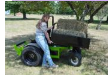
The manual Dump Box is easily lifted to dump its contents.
